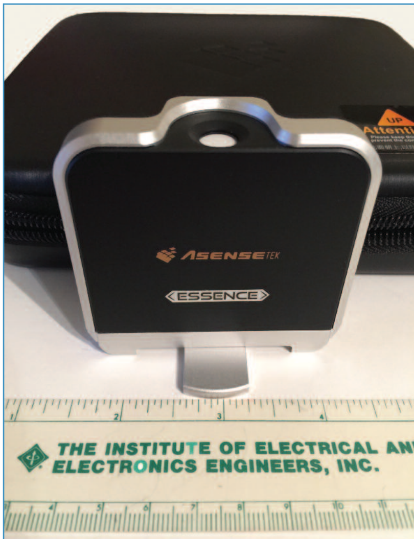
The Asensetek Lighting Passport light sensor can fit in the palm of your hand and connects through Bluetooth to an app on your smartphone or tablet.
